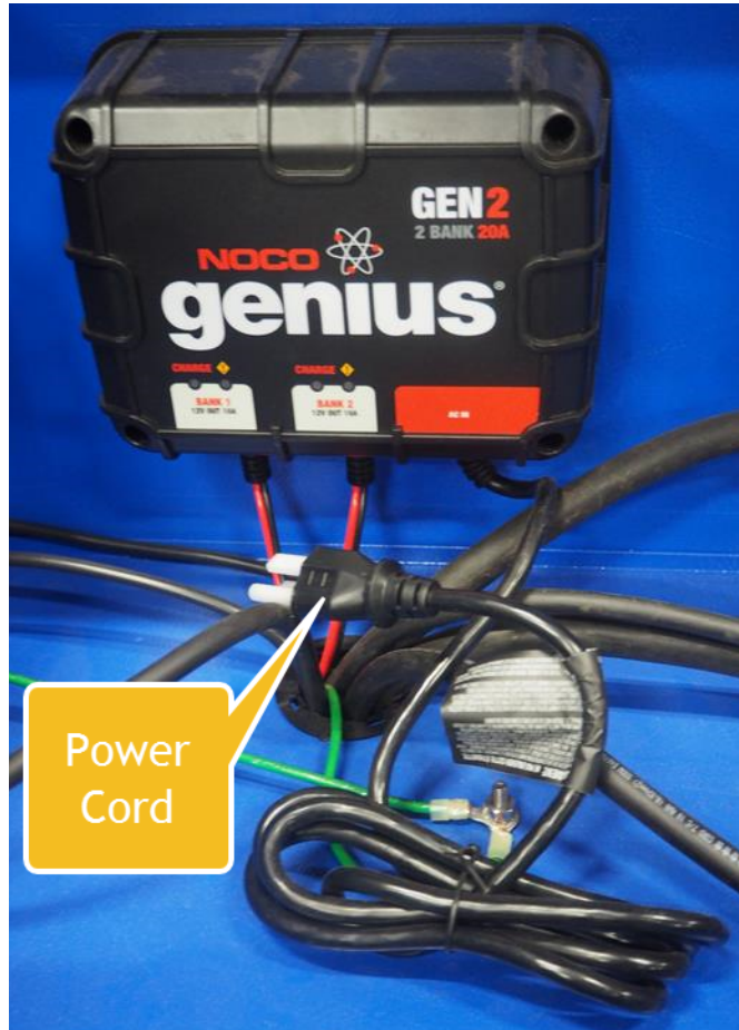
Figure 8: Auxiliary charger module
